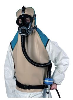
The **ACS 951** face piece is provided with two exhalation valves protected by special caps, two ducts moulded into the face piece lead the air to skim the lenses thus preventing steaming up. The lenses are double (external part in glass and internal part in polycarbonate) and easily replaceable. The harnesses are external and fixed to the face piece by means of self adjusting buckles for quick and easy donning. The hood is sewn onto the mask and protects the wearer down to the waist
